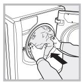
Quilts: to wash quilts with a synthetic outer layer, use the bag provided and set the wash cycle to  $\triangle$ .
